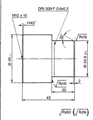
Improvised clamping pin for drive spindle with multi-plate clutch
